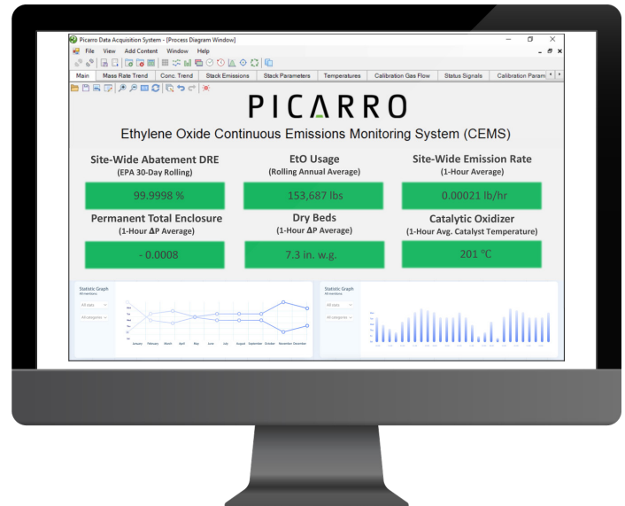
Figure 2: The Picarro CEMS features a live dashboard of stack emissions for improved confidence in emissions control.
