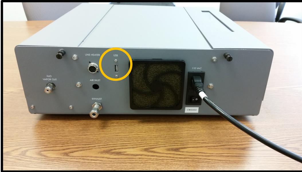
Figure 4: Rear of the CWS with the USB port highlighted in yellow.
