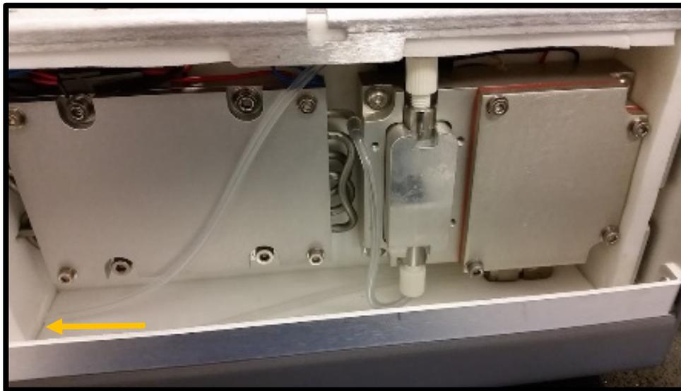
*Figure 29: Route the outlet tube via the indent on the left side of the membrane housing.*
