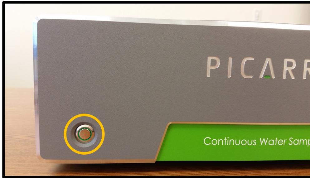
*Figure 8: Power button on front of CWS is off (no light).*
