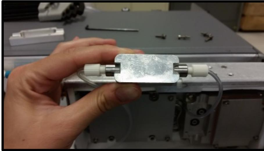
Figure 26: Photo of the membrane removed from the housing. Once it is out of the housing, it is easy to unscrew the tubing connections and replace the cartridge.
