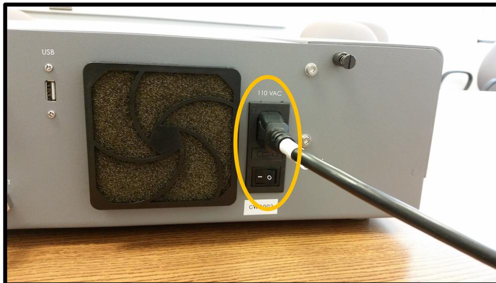
Figure 5: Rear of the CWS with power switch and cable. The power switch is "On" in this image ("I" is depressed).
