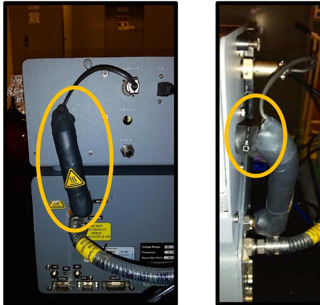
Figure 2: Rear of the CWS with the transfer line connected between the CWS and the analyzer (left). In addition, a small piece of foam is zip-tied around the upper Swagelok connector (right) to reduce the possibility of a cold spot in the transfer of H<sub>2</sub>O from the CWS to the analyzer.
