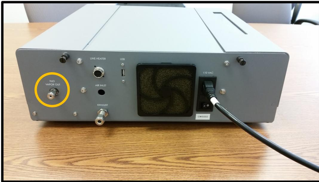
Figure 1: Rear of the CWS with H<sub>2</sub>O Vapor Out port highlighted in yellow.
