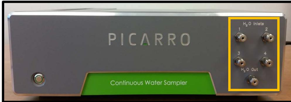
Figure 6: Front of the CWS with the four inlet ports and one outlet port highlighted in yellow.
