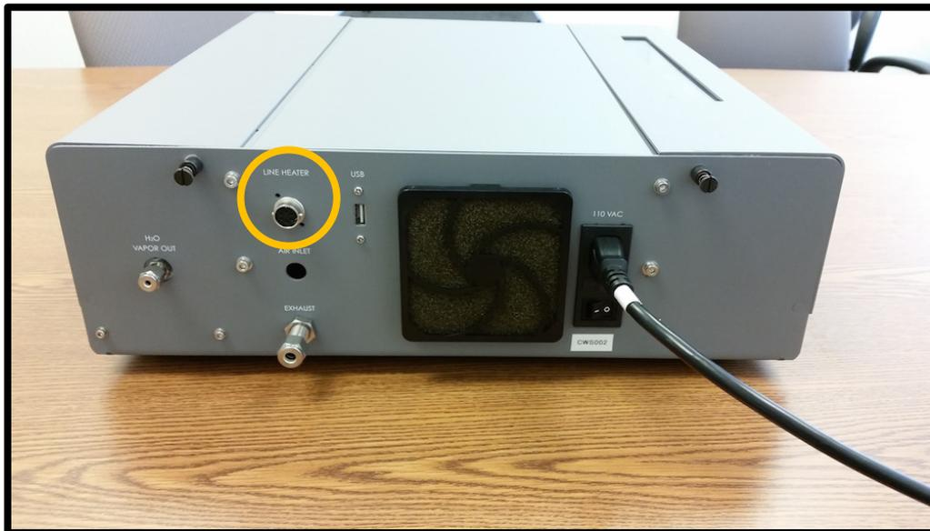
Figure 3: Rear of the CWS with Line Heater quick connect highlighted in yellow.
