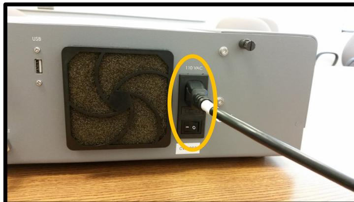
Figure 21: Turn off the mains power by depressing the power switch.
