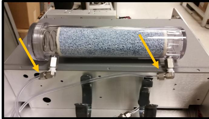
Figure 20: The two highlighted Swagelok connections should be loosened to remove and replace the Drierite.
