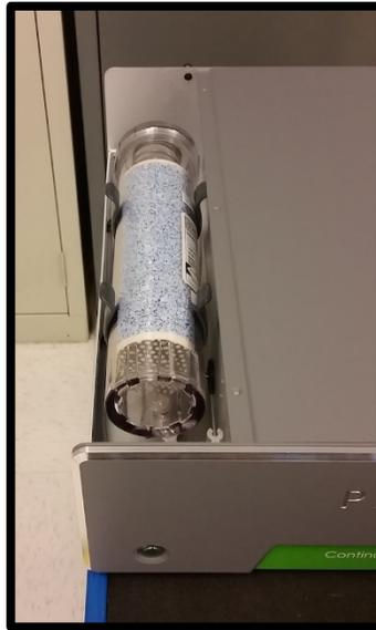
Figure 18: Drierite column with the CWS left top-to-side panel removed.
