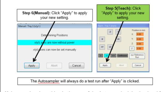
Make sure there's nothing in the way of the Autosampler injection head for this test run.
