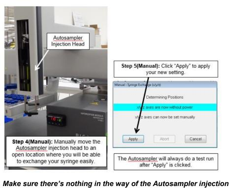
lake sure there's nothing in the way of the Autosampler inject head for this test run.
