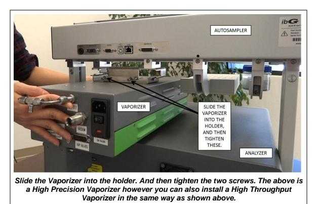
**Continuation of Step 7:** Align the gas delivery line of the vaporizer to the analyzer's gas inlet port by adjusting the location of the vaporizer along the Autosampler. You may need to move the tray and the station holders to make room for the vaporizer. When satisfied with the location of the analyzer and the holders, tighten the screws that connect them to the Autosampler. See images below for more information.
