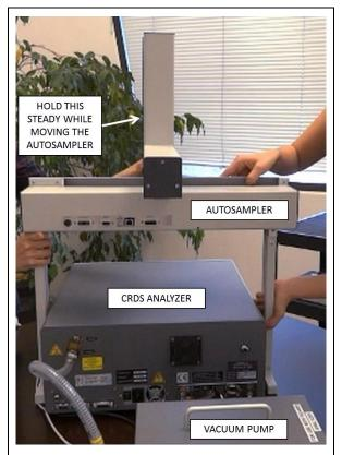
Step 5: Adjust the location of the two legs so that they hug the analyzer.
