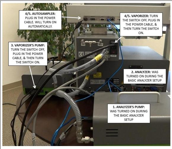
Follow the numbers above to turn on the modules in the correct order. General Rule is to always turn on the pump first. The order of turning on the Autosampler & Vaporizer can be interchanged.
