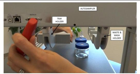
**Step 7:** Set up the vaporizer (**If installing the High Throughput Vaporizer, skip the following Step 7 – Step 12**). First, remove the holder that comes attached to the Vaporizer, and then attach the holder to the Autosampler the same way you had attached the legs to the XYZ arms in the previous steps.
