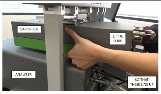
Make sure the screws that attach the holder to the Autosampler are loose while adjusting the location of the vaporizer. To move the vaporizer, lift and slide.
