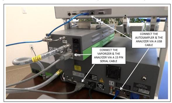
Step 10: Make the cable connections between the Vaporizer and the Autosampler.
