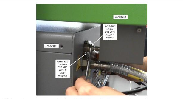
Tighten the connection with the 5/16" and the 9/16" wrench. In practice, the vaporizer and the analyzer should be closer to each other than shown above. A greater space was given in the above image for a demonstration purpose.
