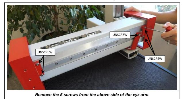
Step 3: Remove the RED metal guards from the XYZ arms by removing the screws.
