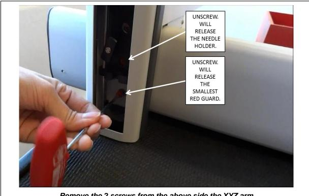
Remove the 2 screws from the above side the XYZ arm
