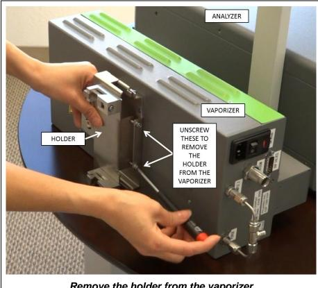
Remove the holder from the vaporizer
