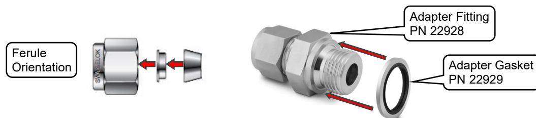
Figure 83: Pump Exhaust Line Adapter Fittings
