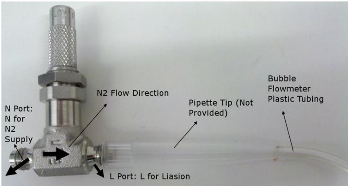
**3.1.7. Use the Pipette Tip to make the connection above (Not Provided)**
