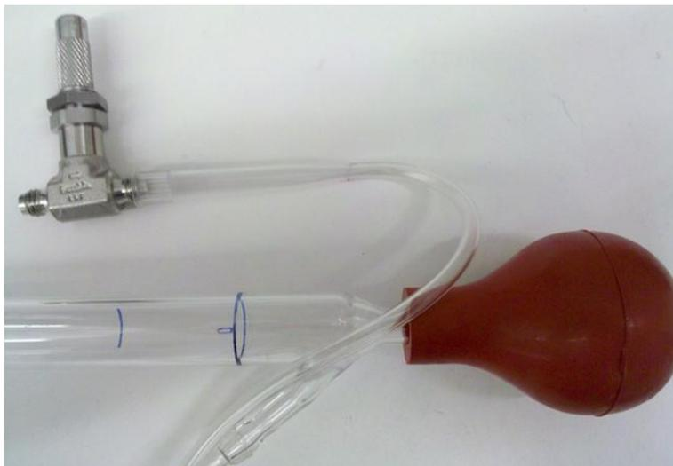
**3.1.6. Connect the Flowmeter to the Needle Valve L Port 70ml/min (Close-Up).**
