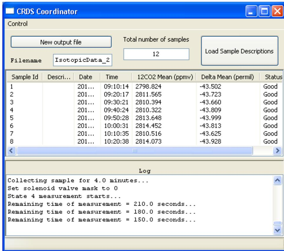
2.4.12. The bottom half of the coordinator window serves as the log/status of all the processes taking place within the Liaison interface during sample analysis. It also displays the error messages when an error occurs.
