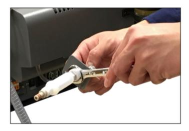
Figure 59 - Removing Filter from Pressure Inlet Bulkhead
