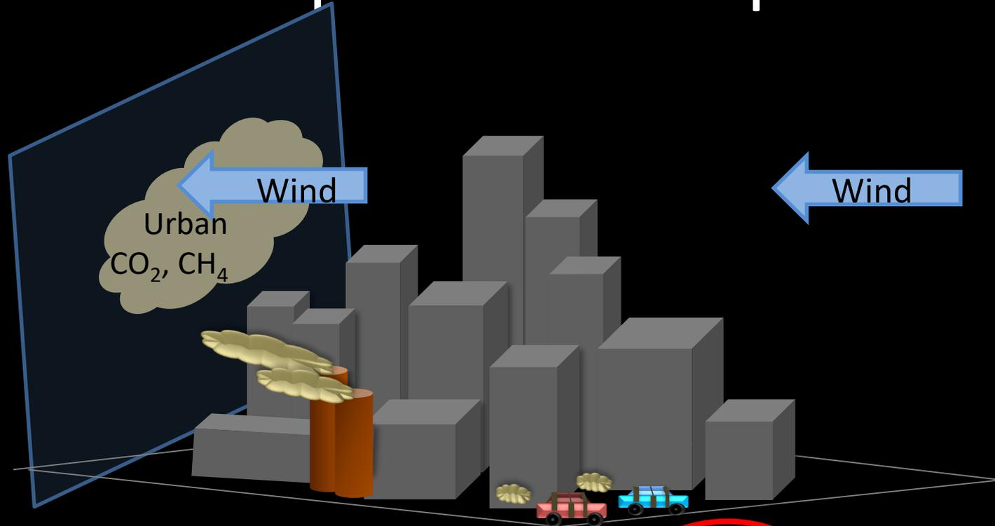
$$F = \frac{\int_0^{z_i} \int_{-x}^x \left( \frac{[C]_{ij} - [C]_b}{1 \times 10^a} \right) \times n_{dij} \times U_{\perp ij} dx dz}{A_{city} \Delta CO_2 \text{ Transport}}$$
