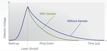
Light intensity as a function of time in a WS-CRDS system with and without a sample having resonant absorbance. This demonstrates how optical loss (or absorption by the gas) is rendered into a time measurement (left). By using a patented wavelength monitor, this
