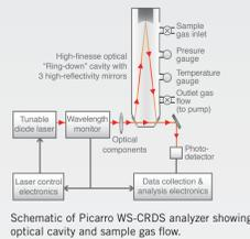
Schematic of Picarro WS-CRDS analyzer showing optical cavity and sample gas flow.
