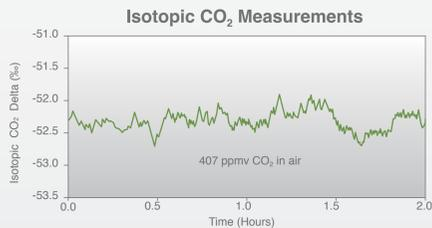
Data from a Picarro isotopic CO<sub>2</sub> analyzer measuring the isotopic carbon (<sup>13</sup>C/<sup>12</sup>C) ratio from a constant-concentration (407 ppmv) CO<sub>2</sub> gas stream. The measurement precision is 0.15 per mil (in δ<sup>13</sup>C units) in a 5-minute measurement.
