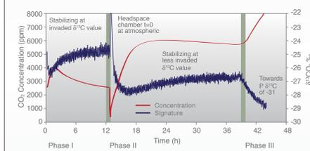
Soil chamber measurements of concentration and isotope ratio subject to apparatus in different configurations. Raw delta data without smoothing.
