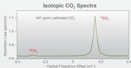
CO<sub>2</sub> spectrum taken by Picarro analyzer showing the extremely high measurement resolution (0.0001 cm<sup>-1</sup>). Carbon isotope ratios are calculated by measuring the relative concentrations of the two isotopologues of CO<sub>2</sub>.
