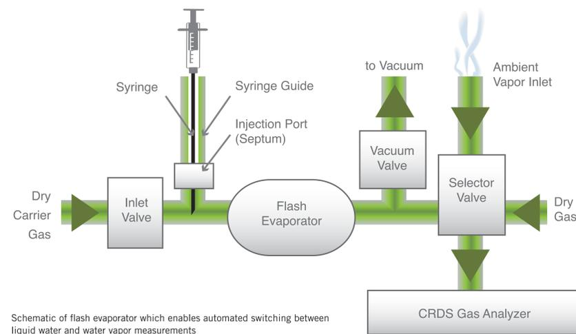
Schematic of flash evaporator which enables automated switching between liquid water and water vapor measurements
