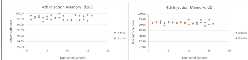
For DI water, the memory performance is stable, just as in the case when no SL is implemented.
