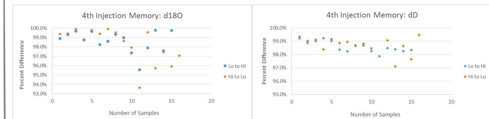
For 4% TDS seawater samples, the memory performance starts to degrade after 200 injections (~ 30 hr of continuous run), suggesting that the SL needs to be replaced or cleaned. The replacement of the SL takes minimum down-time (a few minutes) compared with the time needed to clean the vaporizer chamber (24 hours).
