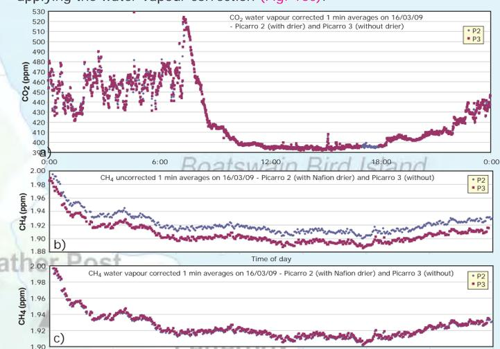
Fig. 10 - Water vapour corrections applied to data for Picarro 2 (dried air) and Picarro 3 (undried), a) application of factory CO<sub>2</sub> correction, b) and c) before and after application of the RHUL CH<sub>4</sub> correction.
