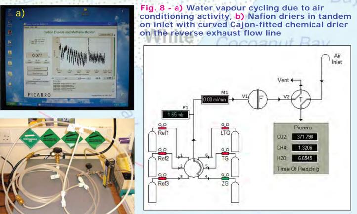
Fig. 8 - a) Water vapour cycling due to air conditioning activity, b) Nafion driers in tandem on inlet with curved Cajon-fitted chemical drier on the reverse exhaust flow line. Fig. 9 - Screen shot of software being developed at UEA for automated flow control, standard analysis and data retrieval
