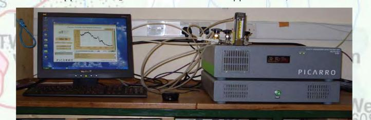
Fig. 7 - Picarro 2 with Nafion drier on the inlet line which tees off from the Dekoron airline seen in the background
