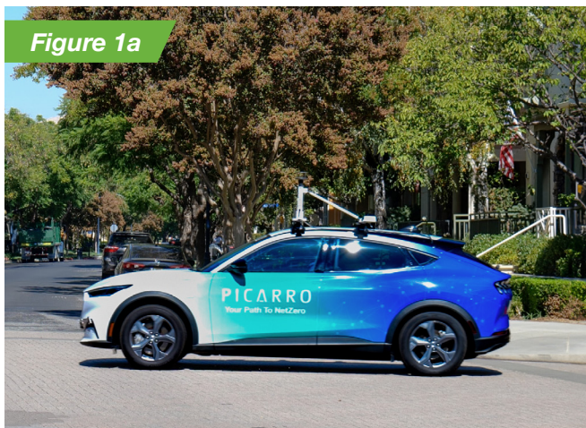
Figure 1. Picarro's solution enables seamless leak detection with both vehicle-mounted (1a) and handheld sensors, ensuring efficient on-foot leak confirmation and repair (1b).
