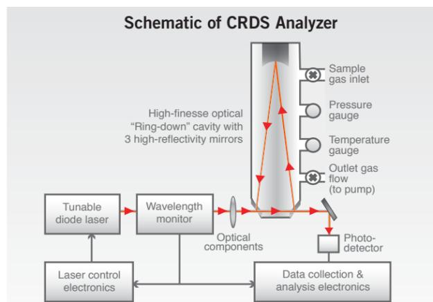
Fig. 4: Schematic of Picarro CRDS analyzer showing optical cavity and sample gas flow.
