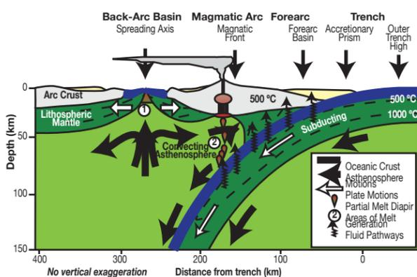
Figure 2: Dehydration of the subducting slab results in mantle melt which erupts forming island arc chains. Back-arc spreading causes a ridge to form in the back-arc basin, similar to a MOR.
