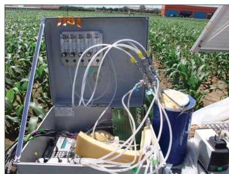
Cryogenic trapping setup and IRGA
